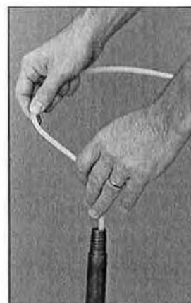
Figure 3. Engaging threads by rotating tubing.
