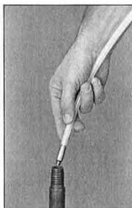
Figure 2. Insertion of tubing and PRT adapter.
