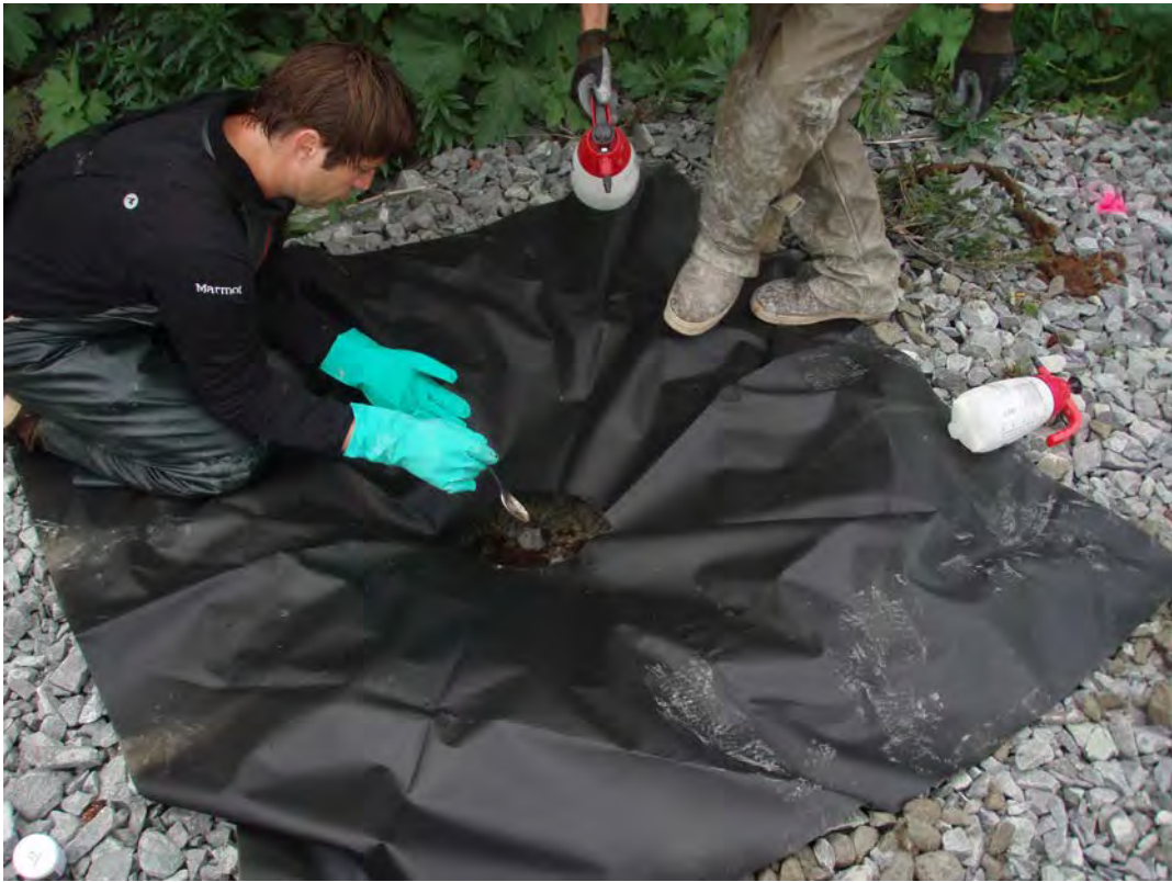
Photo 9: Spray clean spoon, gloves, auger, tarp and bowl with Alconox and water
