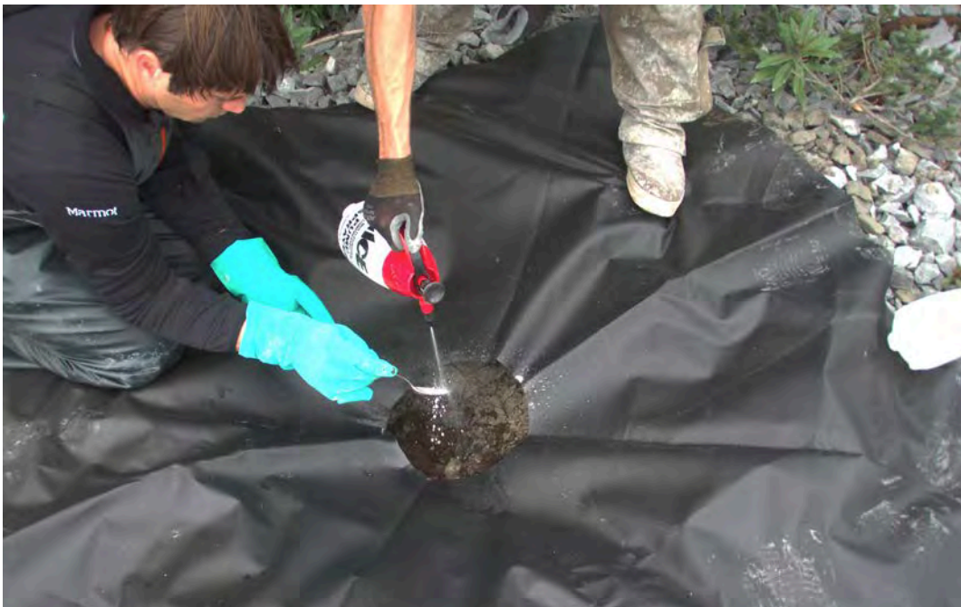
Photo 10: Spray clean spoon, gloves, auger, tarp and bowl with Alconox and water
