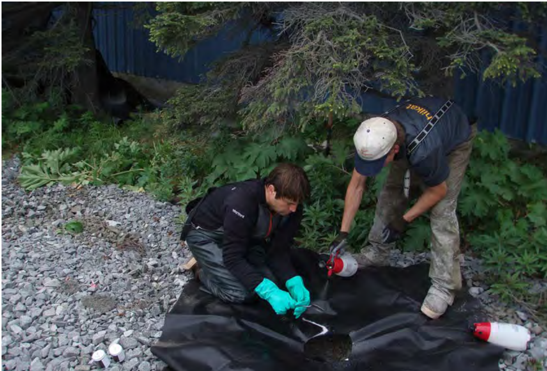
Photo 12: Spray clean spoon, gloves, auger, tarp and bowl with Alconox and water
