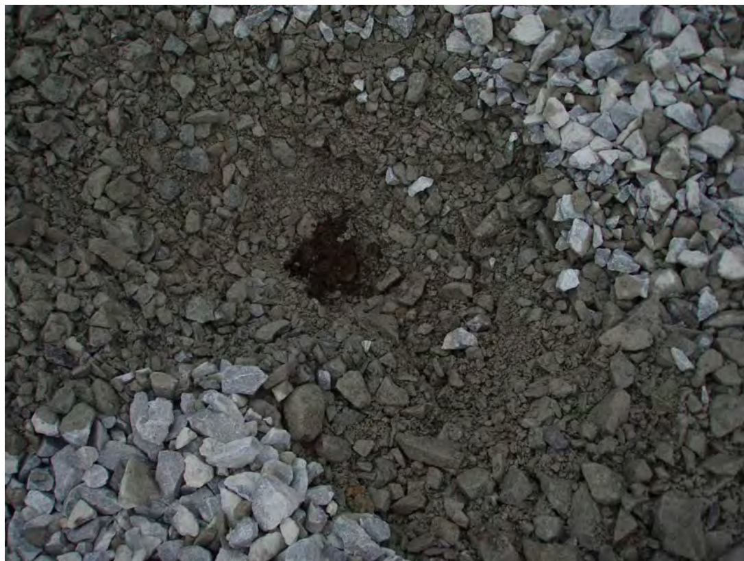
Photo 3: Further expose fine grain soil without redistributing
