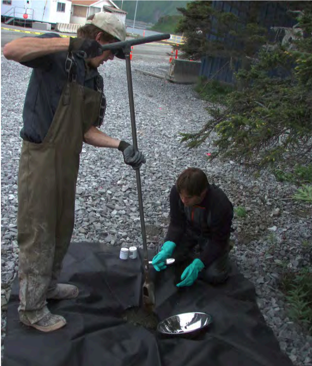
Photo 4: Auger into fine grain soil and store fines in stainless steel bowl.
