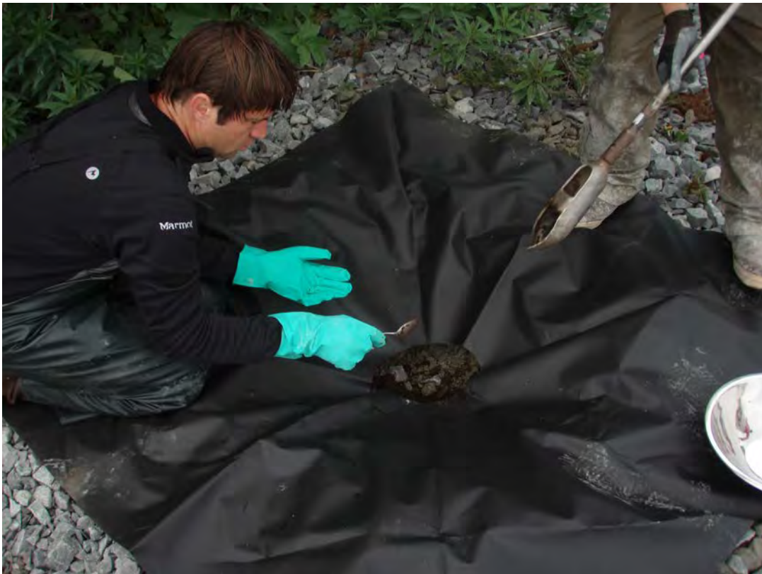
Photo 8: Place fines from bowl into auger pit and use spoon to clean auger of soil
