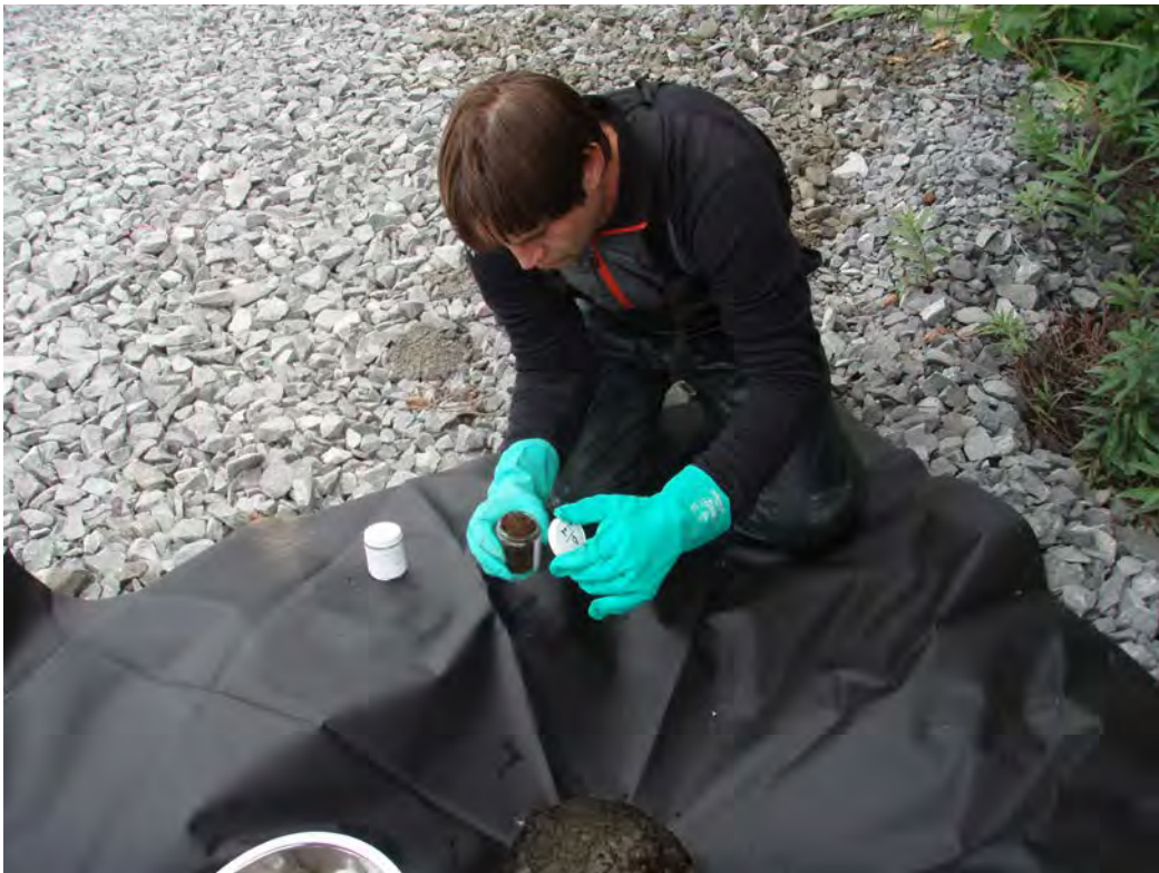
Photo 6: Cap jar over pit to direct spillage
