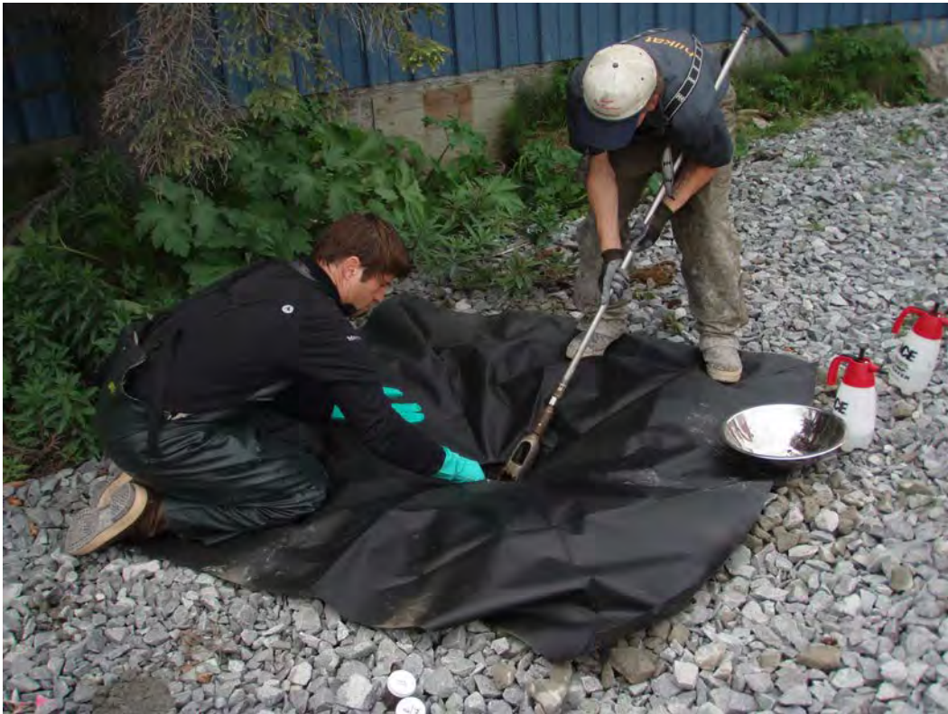
Photo 7: Place fines from bowl into auger pit and use spoon to clean auger of soil
